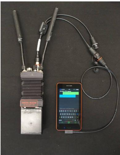
PriveTAK handheld terminal with 4W MESH node
